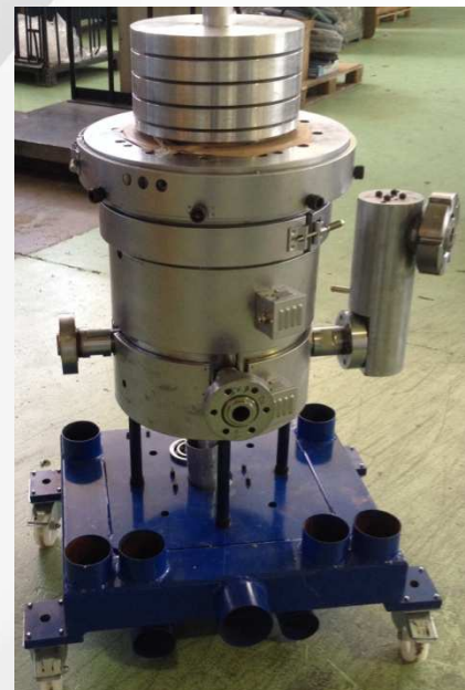
New die head \varnothing 300mm die size Heating 10-15 kWh Steel Weight approx 0,43to
